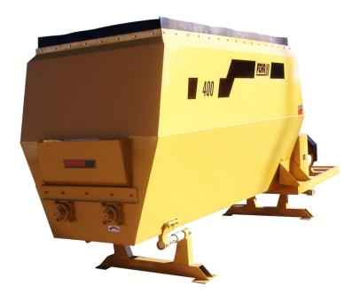
The mixer has a control lever located on the goose to activate the download and distribution of feed in the hopper, you must maneuver a lever to open the door, another to activate the band when you go to deposit the mix in the forage feeders and another to lower or raise the band.
